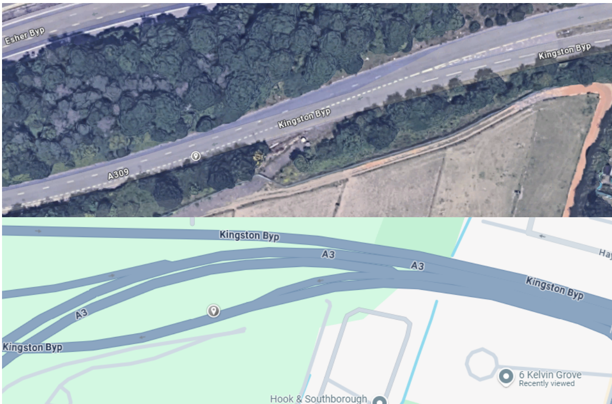
Figure XX Dropped pin marks high point of clash between traffic flows, those decelerating to exit A309 and those accelerating to merge onto A309 from on slip.
